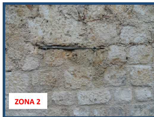
Santa Maria di Collemaggio: double Flat-Jack test to characterize masonry of the wall of the church
